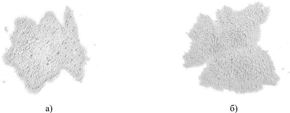
Fig. 1. Structural formations a) and b) in film coatings obtained as a result of carbon deposition using PVD technology
